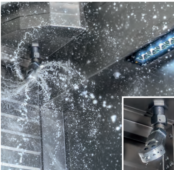
Work area flushing and lighting
