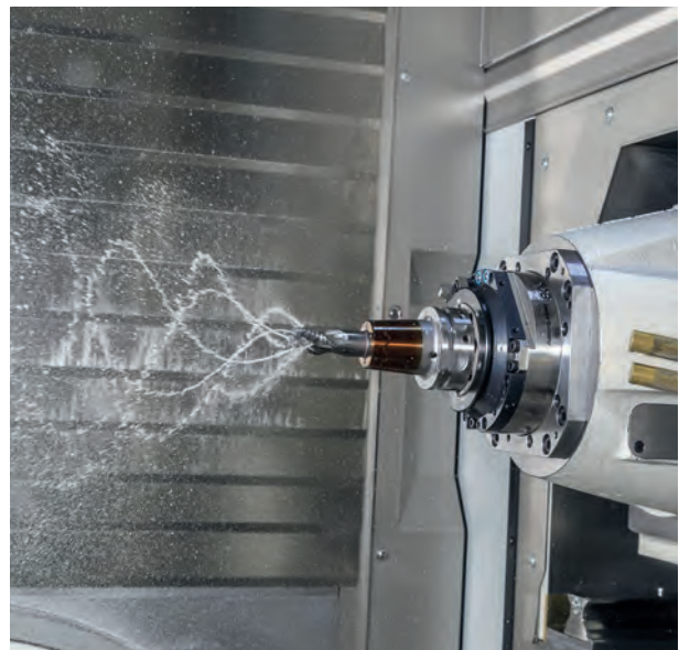
Internal cutting fluid supply (23 bar)
